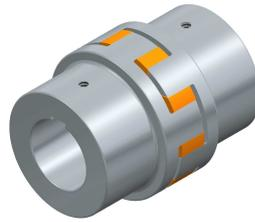
The ELKURI coupling is a torsionally flexible, fail-safe jaw-type coupling and consists of two hubs, between which is fitted an elastic element. The elements are supplied in the shorehardnesses **92, 98 °Shore A and 64 °Shore D** (temperature range -40°C to +110°C). Other shorehardnesses are available on request.
